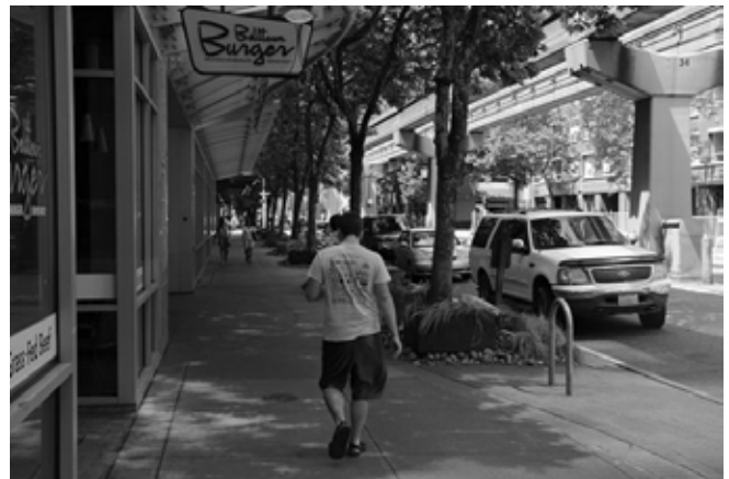
This sidewalk along 5th Ave offers an example of a well-maintained pedestrian clear zone. Signs, bike racks and plantings are located within the furnishing/landscape zone, and the pedestrian clear zone is unobstructed.
