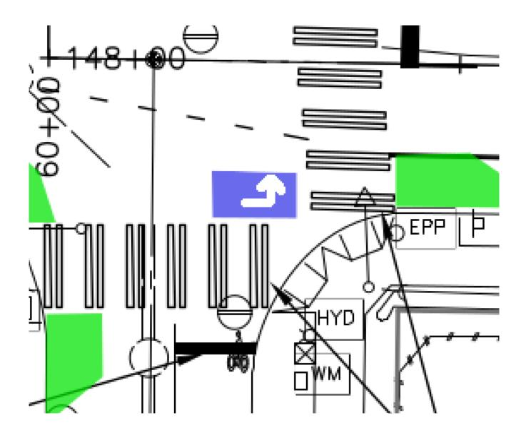
5) **The bus stop at 12<sup>th</sup> Ave NE should have a proper island** rather than conflicting with the bike lane, and the **left turn signal phase (onto 12<sup>th</sup>) should not overlap with oncoming traffic**.
