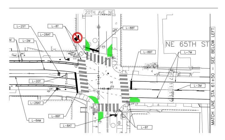
As an aside, the southeast curb bulb in this picture creates a safe space for eastbound cyclists to make a two-stage left turn onto 20<sup>th</sup> Ave NE. A potential enhancement (in purple) is below.
