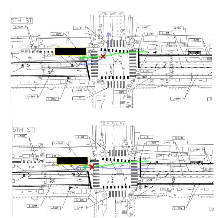
Removing the overlapping left turn phase will eliminate the left-hook risk. Creating a proper bus island will eliminate the risk of getting hit from behind (or getting hit by a bus pulling in or out of the stop).
